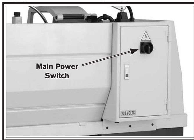
Figure 23. Location of the master power switch.
